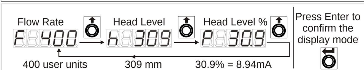
**If Totalizer is enabled by selecting Flow Rate time base unit**
